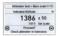
For each set point, the operator adjusts the altimeter's barometric scale to the commanded "Set scale" value, and compares the altimeter reading to the measured value on the instrument.
