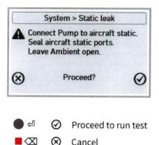
This page provides recommended configuration of the aircraft and instruments under test and waits for an acknowledgement that the operator has completed this configuration before proceeding with the test. If the aircraft and instruments cannot be safely configured for the test, the operator should cancel the test.
